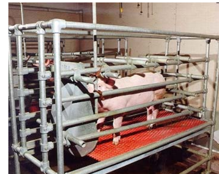
Intact pig housed in a metabolic tubular crate for short-term collection of faeces and urine
