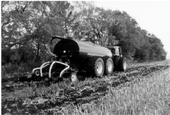
Figure 7. Low or high disturbance liquid manure injection system using a tool bar mounted on a tanker (Source: PAMI, 2002).
