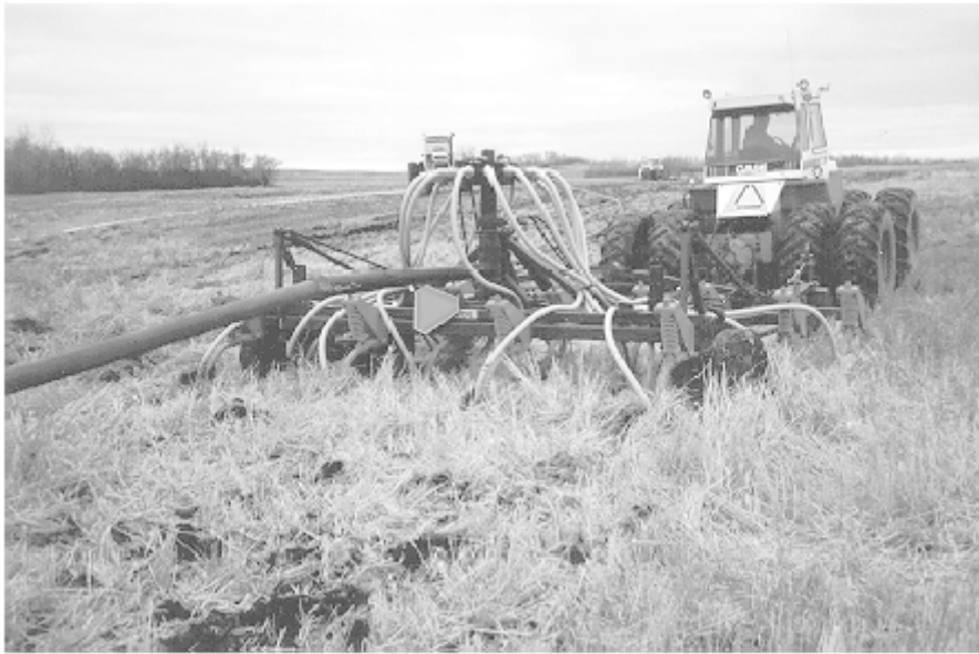
Figure 6-a. Pipeline manure injection system using drag hose connected to manifold distributor on chisel plow-based tool bar (Source: PAMI, 1997a).
