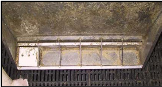
Figure 1. Feeder trough coverage with a gap adjustment providing a gap opening of 9.2 mm.
