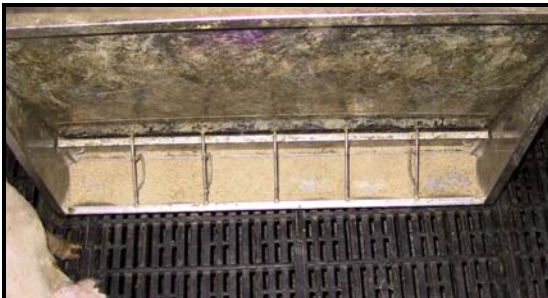
Figure 3. Feeder trough coverage with a gap adjustment providing a gap opening of 31.5 mm.
